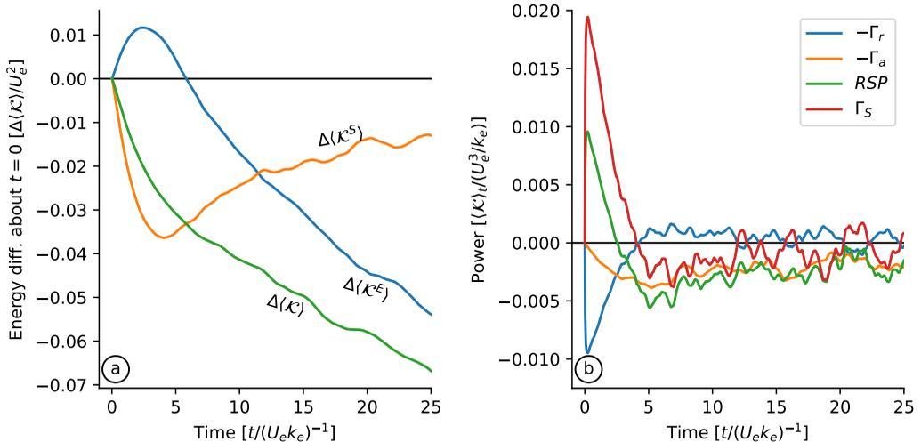
FIGURE 13. Diagnostics of the 2D turbulence solution with parameters presented in table 4. (a) Kinetic energy change about initial condition. (b) Refractive and advective conversion terms, and shear production.
