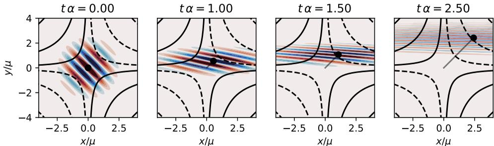
FIGURE 10. The escape of a Gaussian near-inertial wave packet from the saddle of a strain flow. The Gaussian decay scale is  $\mu = \nu$ . The waves are weakly dispersive:  $\hbar = \eta/\alpha\mu^2 \approx 0.1$ . Black contours show the streamfunction  $\psi = -\alpha xy$ , and colors represent wave zonal velocity; the colorbar limits are fixed. The black dot indicates the center of the packet and the gray line tracks its trail.
