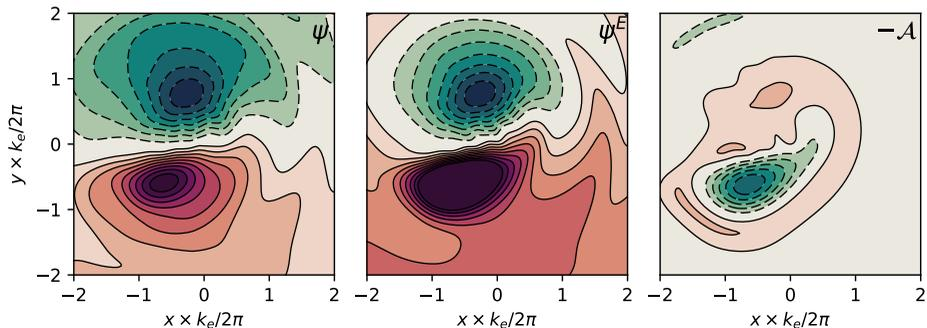
FIGURE 12. Snapshot of the dipole Lagrangian-mean streamfunction and its decomposition into Eulerian-mean and Stokes drift. The snapshots are at  $t \times U_e k_e = 10$ , just after the end of the refractive stage. The spatial average of each field was removed for direct comparison.
