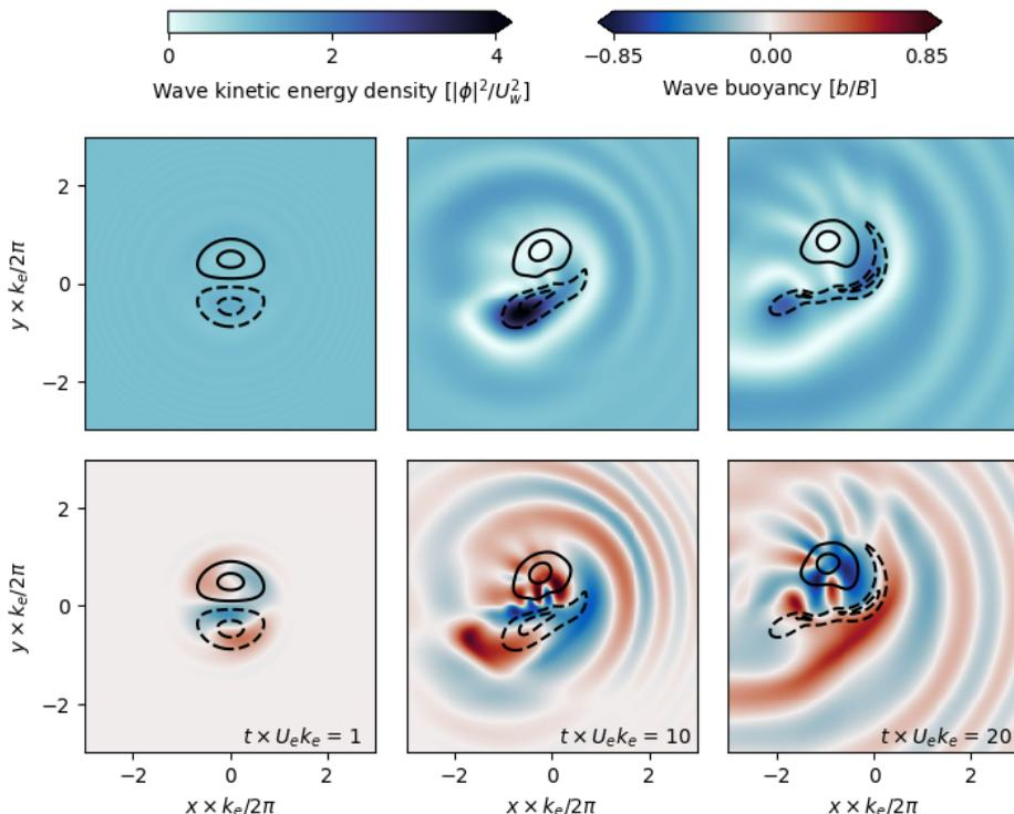
FIGURE 1. Snapshots of the Lamb-Chaplygin dipole solution with parameters presented in table 2. Contours depict potential vorticity,  $q/(U_e k_e) = [-1.5, -0.5, 0.5, 1.5]$ , with dashed lines showing negative values. The upper row shows the wave action density  $|\phi|^2/2f_0$ . The lower row shows the wave buoyancy; the buoyancy scale is  $B = k_e m U_w f_0 \lambda^2$ . These plots only show the central  $(1/5)^2$  of the simulation domain.
