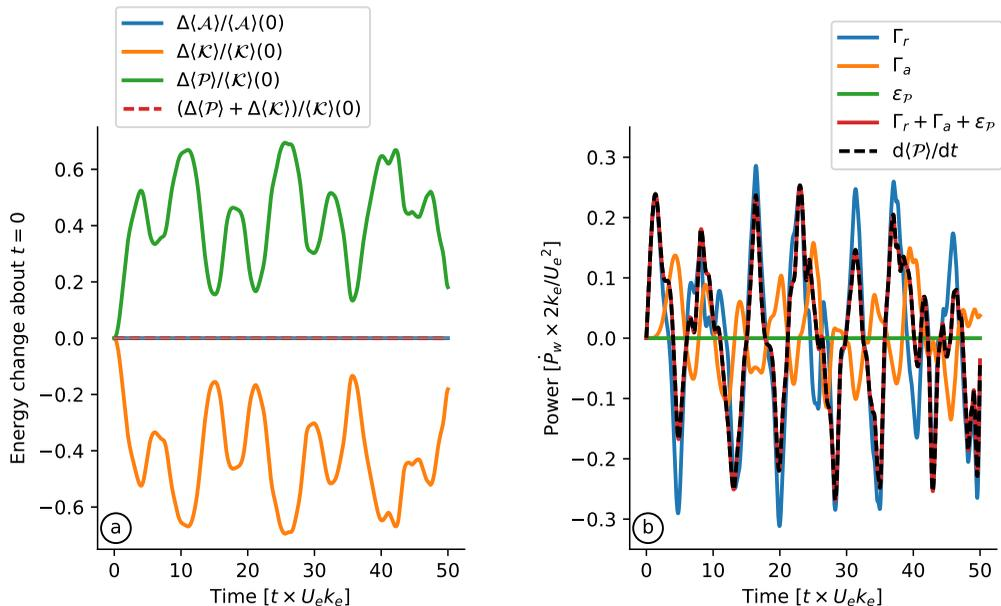
FIGURE 14. Diagnostics of an illustrative solution with initially uniform wave and  $\psi(t=0) = \sin x + \sin y$ , with  $\alpha = 0.1$  and  $\bar{h} = 2$ . (a) Energy difference about initial condition. (b) Wave potential energy budget.
