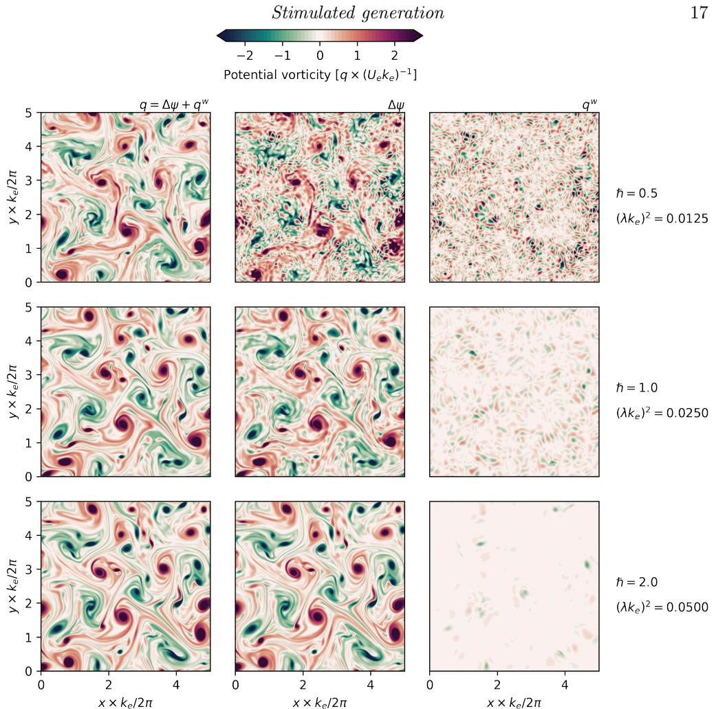
FIGURE 7. Snapshots of PV  $q$  and its decomposition into relative vorticity  $\zeta = \Delta\psi$ , and wave potential vorticity  $q^w$ . The snapshots were taken at  $t \times U_e k_e = 25$ .
