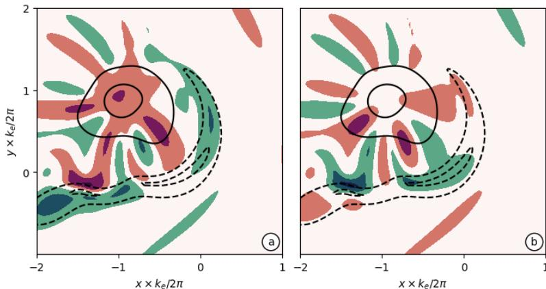
FIGURE 2. (a) Snapshot of  $q$  (contours) and  $\zeta$  (colors) at  $t \times U_e k_e = 20$ . (b) Snapshot of  $q$  (contours) and wave PV  $q^w$  (colors). Both black lines and colors depict the contour levels  $[-1.5, -0.5, 0.5, 1.5] \times (U_e k_e)$ . Solid lines and reddish colors depict positive values; dashed lines and greenish colors show negative values.
