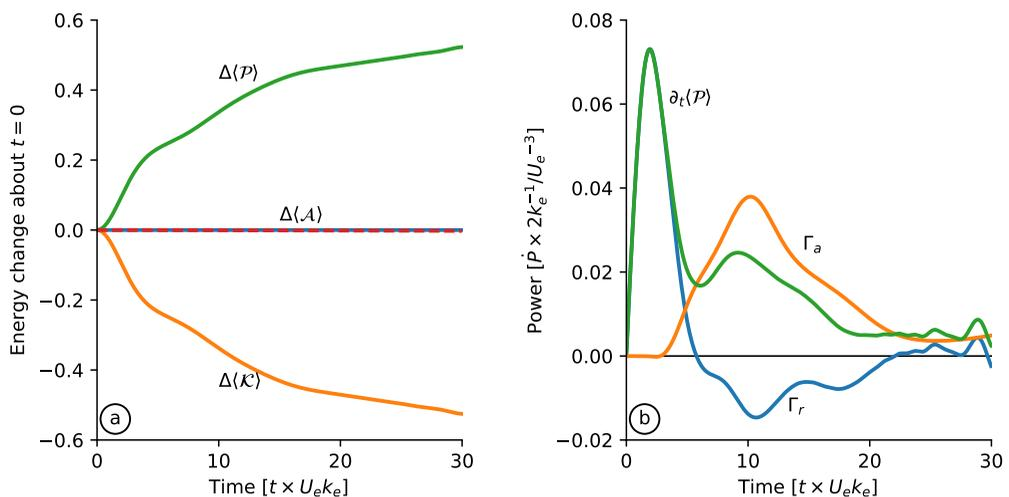
FIGURE 4. Diagnostics of the Lamb-Chaplygin dipole solution with parameters presented in table 2. (a) Energy change about initial condition. (b) Wave potential energy budget (3.12).
